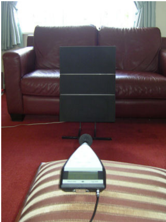
Calibrated mic 4 ft. from speaker
