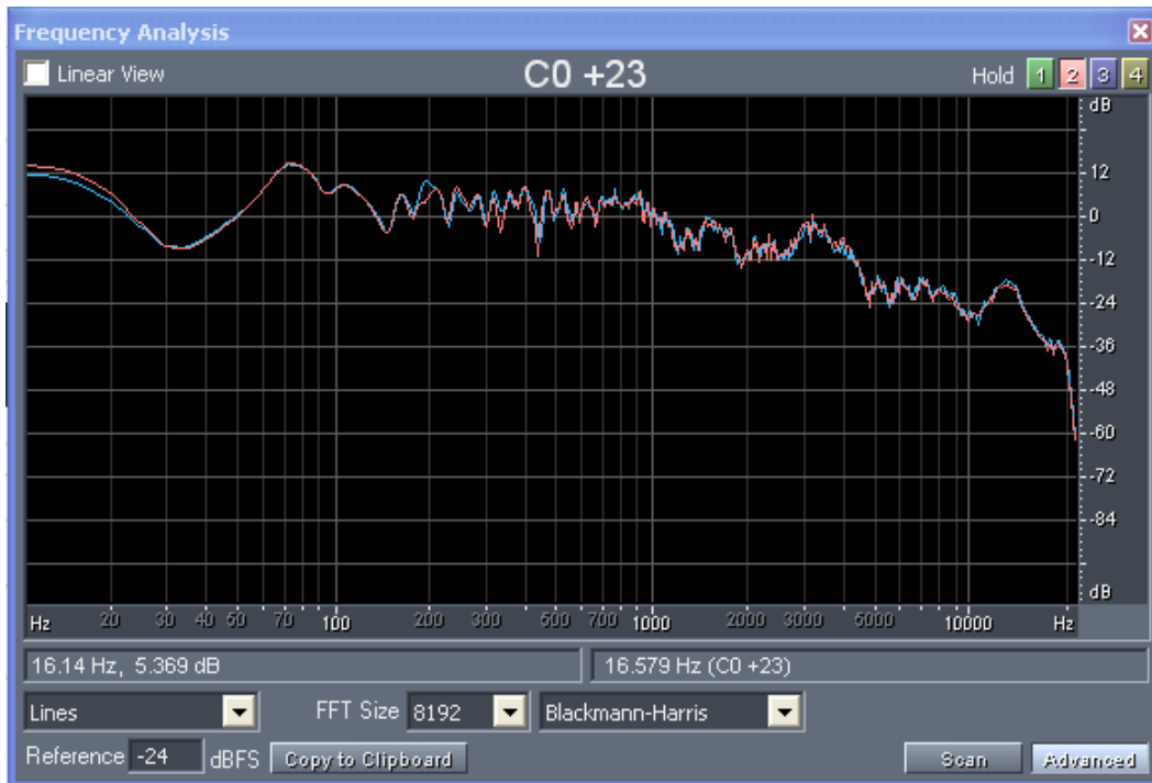
Speaker 1 – before (Red) and after (Blue) 10sec burst of Pink Noise
