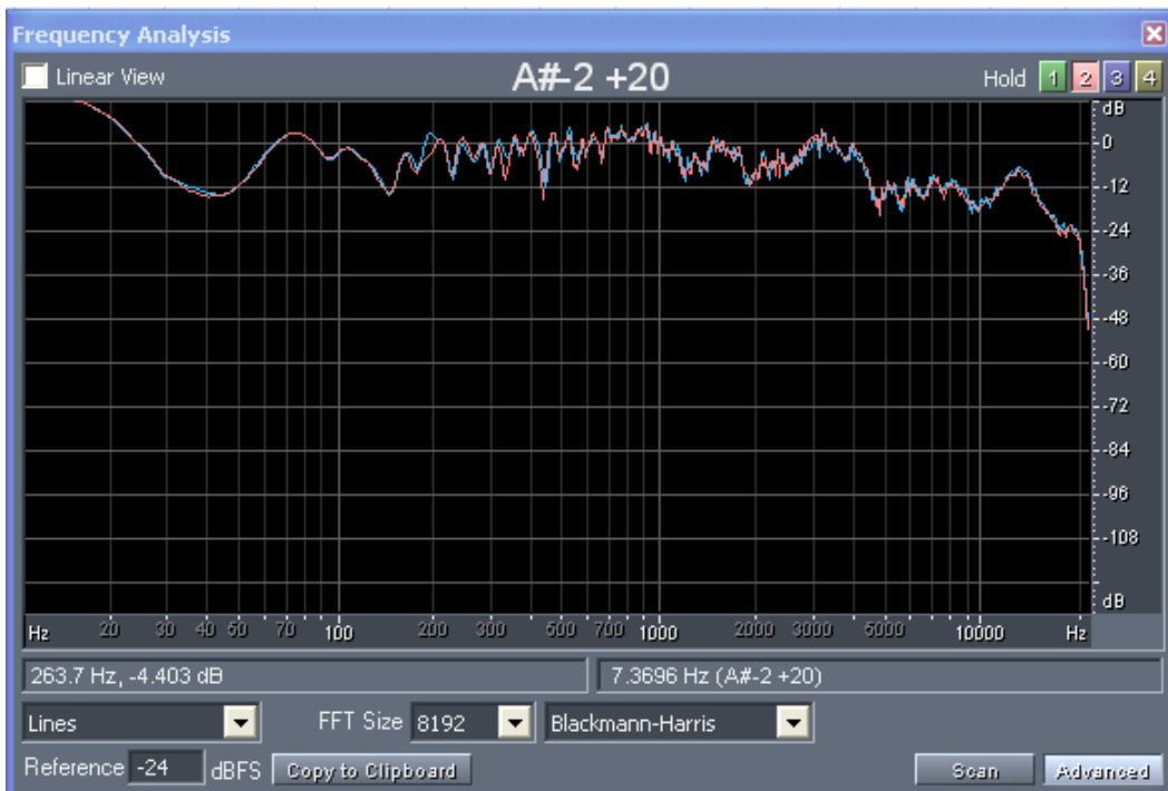
Speaker 1 – before (Red) and after (Blue) 10sec burst of White Noise
