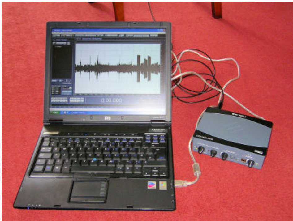
Recording Equipment – HP laptop & EMU 0202 Audio Interface
