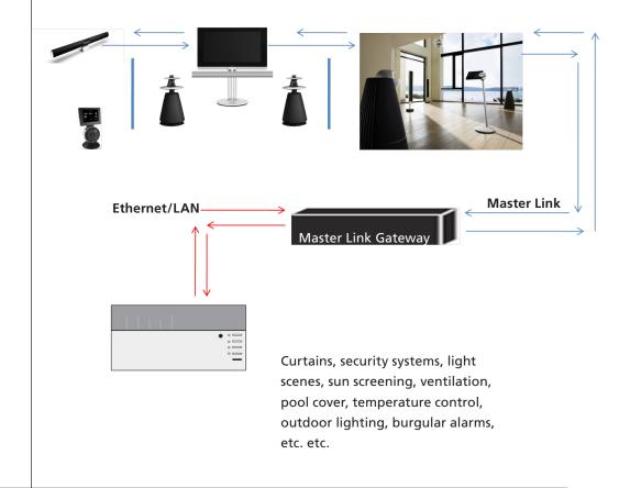
The Master Link Gateway translates the Bang & Olufsen Master Link commands into RS232 or LAN (ethernet) commands that Home Automation can understand and vice versa. The connection varies according to the specifications of the third party product:
